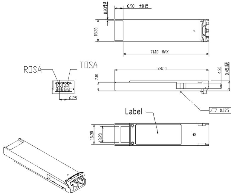
Figure3. Mechanical Specifications
